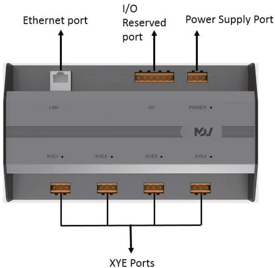
The IMMP-BAC(A) has four M-net ports (XYE), one Ethernet cable port, a power port and a power switch. It connects the MDV CAC Central Air Conditioning system with the M-Net ports and connects the local area network or Internet with Ethernet port. It uses a browser on computer or other similar devices to access the IMMP-BAC(A) websites to monitor the VRF units and do the required settings to connect the IMMP-BAC(A) with the IMMPRO or BACnet BMS software.
