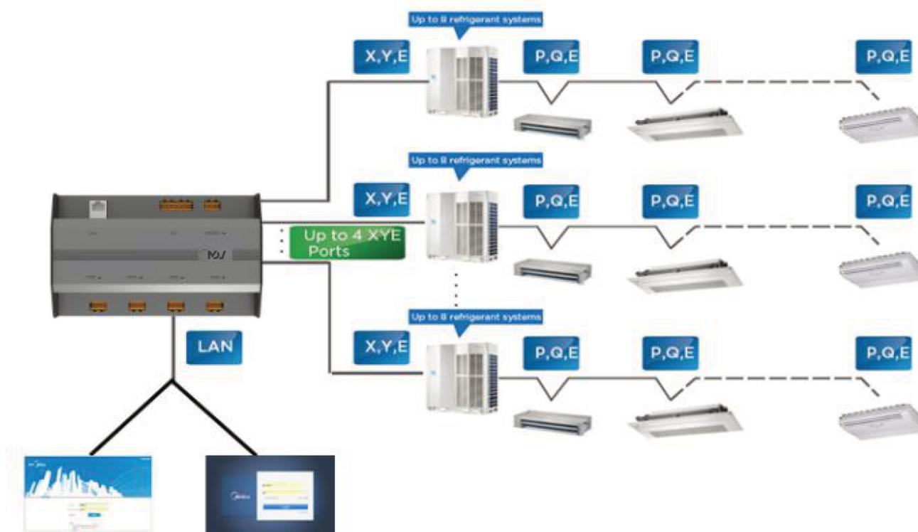
4 M-Net(485A~485D) ports are used to connect to the air conditioners. On each XYE port of the IMMP-BAC(A) the maximum number of indoor units that can be connected is 64 whereas the maximum number of outdoor units that can be connected is 32 outdoor units. Taking all of this in account, the maximum number of indoor and outdoor units that can be connected with 1 IMMP-BAC(A) can be up to 384.
